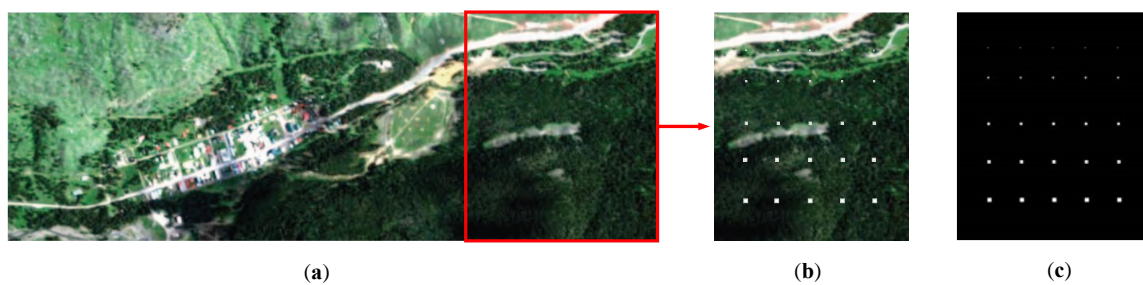
Figure 4. Dataset of synthetic targets for experiment. (a) False color image of the whole scene; (b) false color image of the detection area; (c) ground-truth of simulated dataset.
