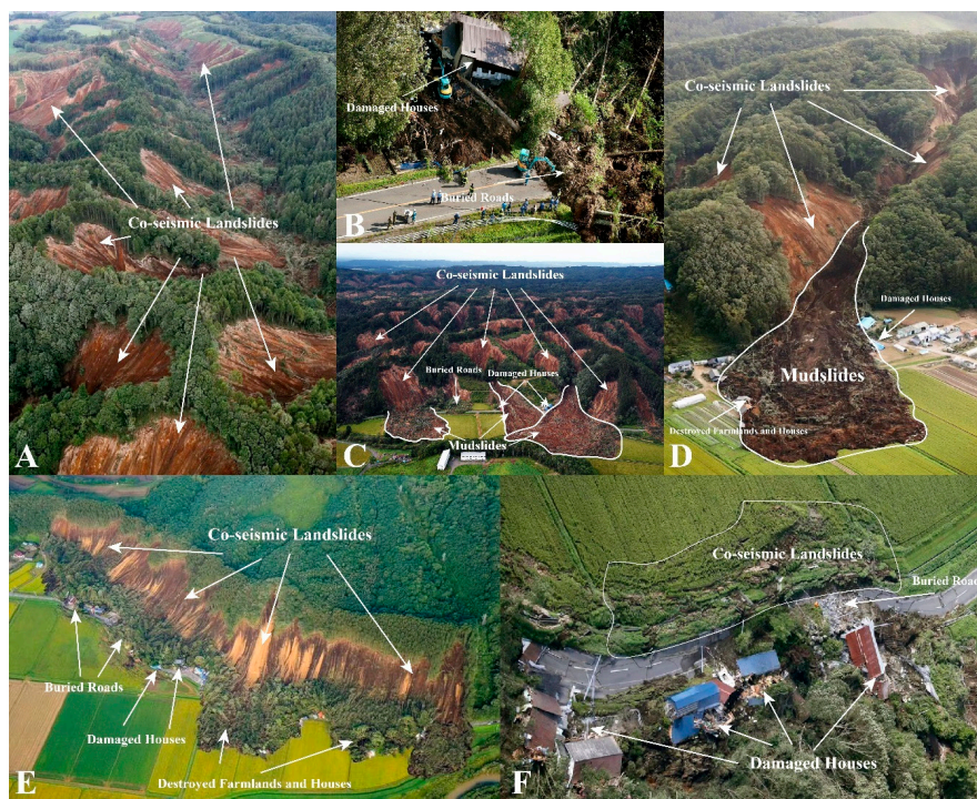
Figure 2. Aerial photos of co-seismic landslides, damaged houses, buried roads and destroyed farmlands and houses in the affected area of the 2018 Ibuli earthquake, taken by Asia Air Survey and Aero Asahi Corporation [52]).
