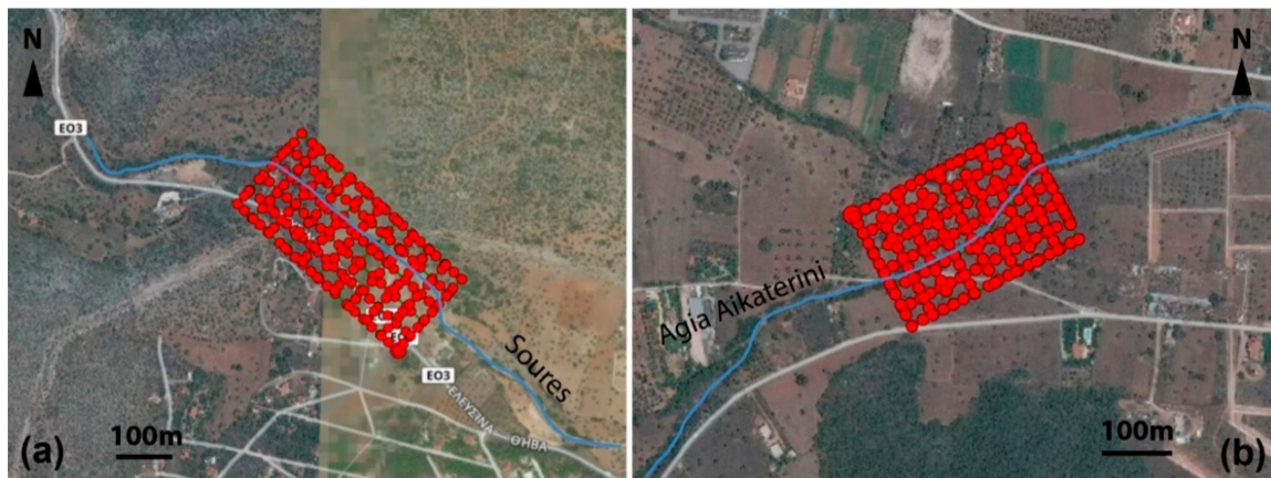
Figure 2. Flight plans for (a) Soures and (b) Agia Aikaterini, with the location of 228 and 226 images, respectively.
