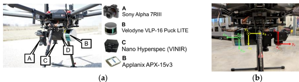
Figure 2. The unmanned aerial vehicle (UAV)-based mobile mapping system used in this study: (a) the sensors mounted on the UAV and (b) the orientation of the global navigation satellite system/inertial navigation system (GNSS/INS) body frame (yellow), laser unit frame (green), and RGB camera frame (red) coordinate systems.
