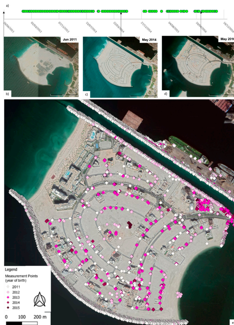
Figure 11. Changes in the studied area over time. (a) Temporal distribution of satellite SAR images. (b) The studied area in June 2011 (from Google Earth, Landsat image). (c) The studied area in May 2014 (from Google Earth, Landsat image). (d) The studied area in May 2016 (from Google Earth, Landsat image). (e) Temporary Measurement Point (MP). The colors identify the year of birth of the MPs. These results are derived using COSMO-SkyMed® PRODUCTS, © ASI (Italian Space Agency)—provided under license of ASI.
