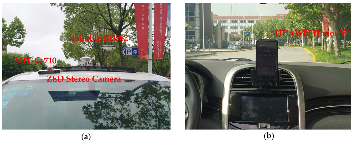
Figure 5. The setup of the kinematic experiment using integrated positioning; (a) integrated navigation vehicle experiment; (b) Huawei Honor V9 placed in the carriage to receive satellite signals.
