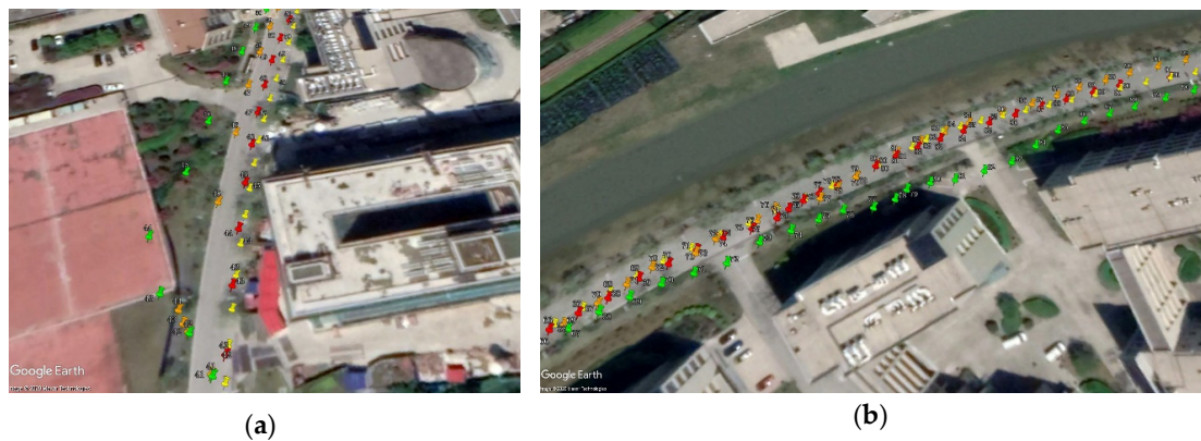
Figure 12. Performance of different Kalman filtering positioning results in shelter zones: (a) shelter zone 1, with the true trajectory represented by yellow points, the positioning results of the CKF fusion method in the integrated navigation system represented by green points, the positioning results of the CI-RKF fusion method in the integrated navigation system represented by red points, and the positioning results of the PRS-IGG-RKF fusion method in the integrated navigation system represented by orange points; the numbers are the points' index; and (b) shelter zone 2, with the same color and number representations as (a).
