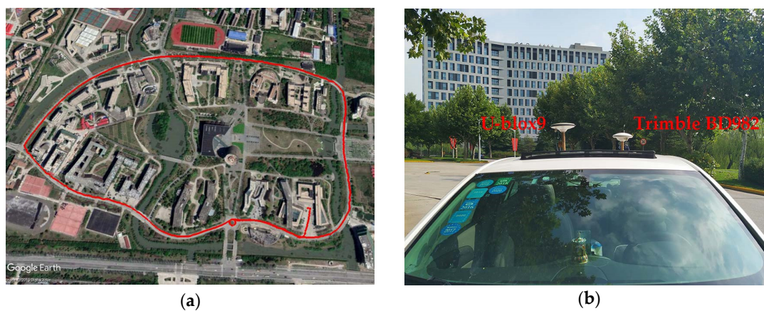
Figure 4. The setup of the kinematic experiment using GNSS positioning; (a) trajectory of the vehicle; (b) onboard equipment for the kinematic experiment.
