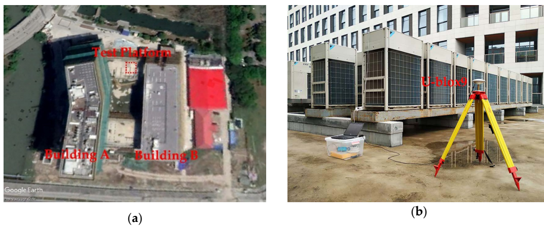
Figure 3. The setup of the static experiment using GNSS positioning; (a) overview of the test platform (marked by the line of dashes) in Google Earth; (b) observation environment of the static experiment.
