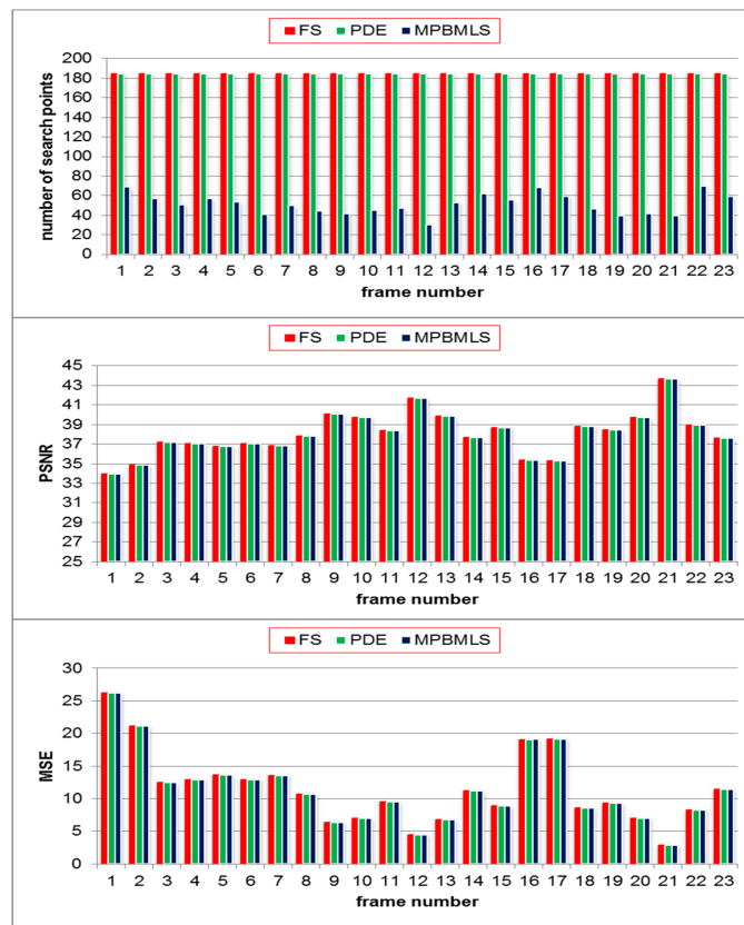
Figure 6. Average number of search points per MB, peak signal-to-noise ratio (PSNR) performance, and mean square error (MSE) of MPBMLS, full search (FS), and partial distortion elimination (PDE) for the “Claire” video sequence of 23 frames.
