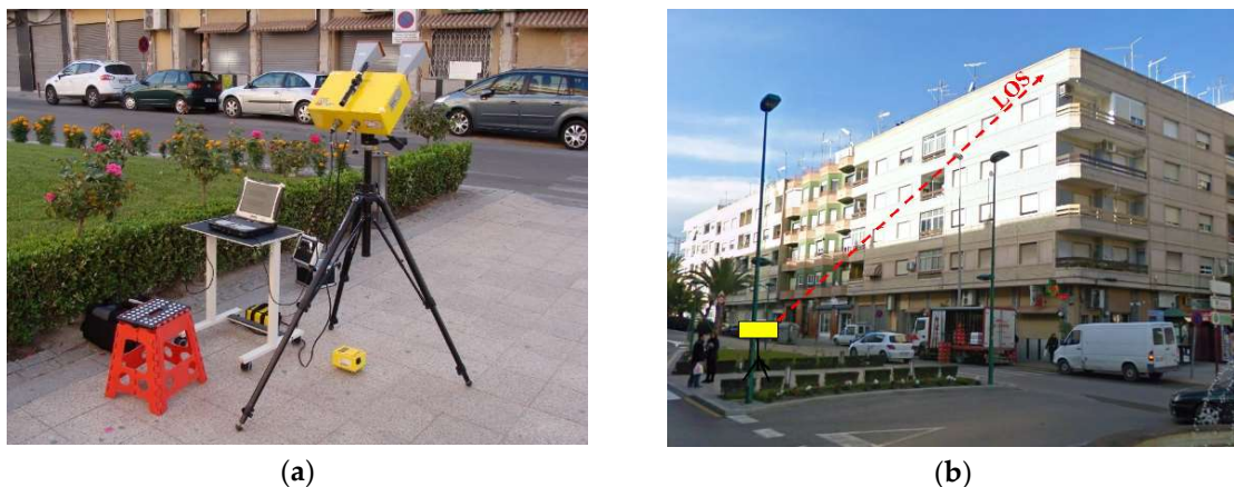
Figure 7. The RAR system (a) performing the remote sensing of the top-west (right) corner of the “La Viña” building (b). The line of sight (LOS), indicated with a red arrow, is in the T direction.
