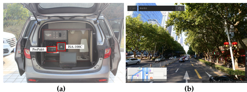
Figure 2. The experimental platform and test environment. (a) shows the data acquisition and calibration equipment, (b) shows a typical lane scenario in downtown Nanjing (from Baidu Map's panorama).
