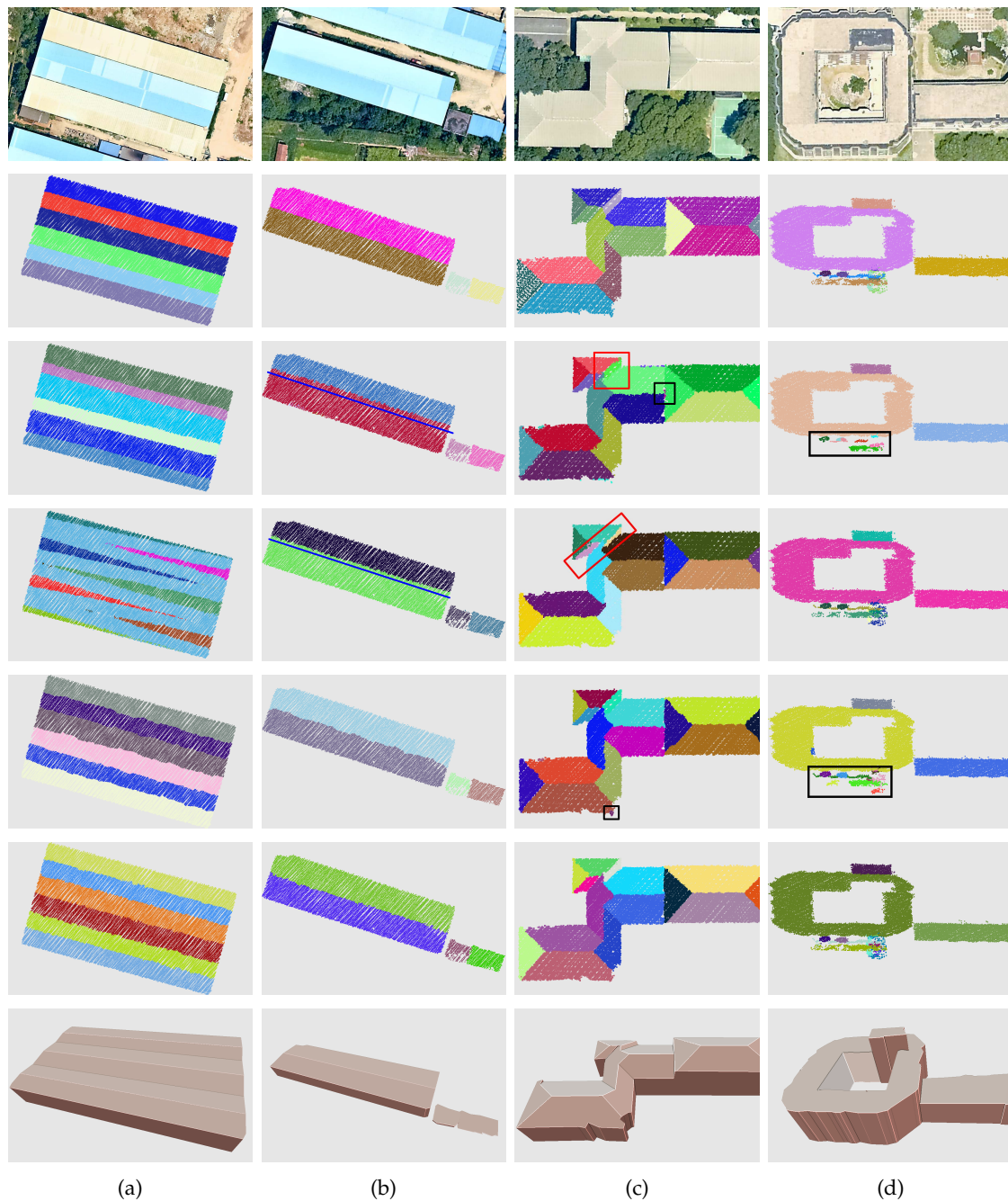
Figure 11. Roof plane segmentation results of different approaches on four local buildings (a–d) selected from the Wuhan dataset. From the first row to the last row: reference images, ground truth, RG, RANSAC, GO, BR, and 3D models. The black rectangles denote the over- or undersegmentation errors and spurious planes. The red rectangles denote the irregular boundaries. The blue lines denote the real boundaries between adjacent roof planes.
