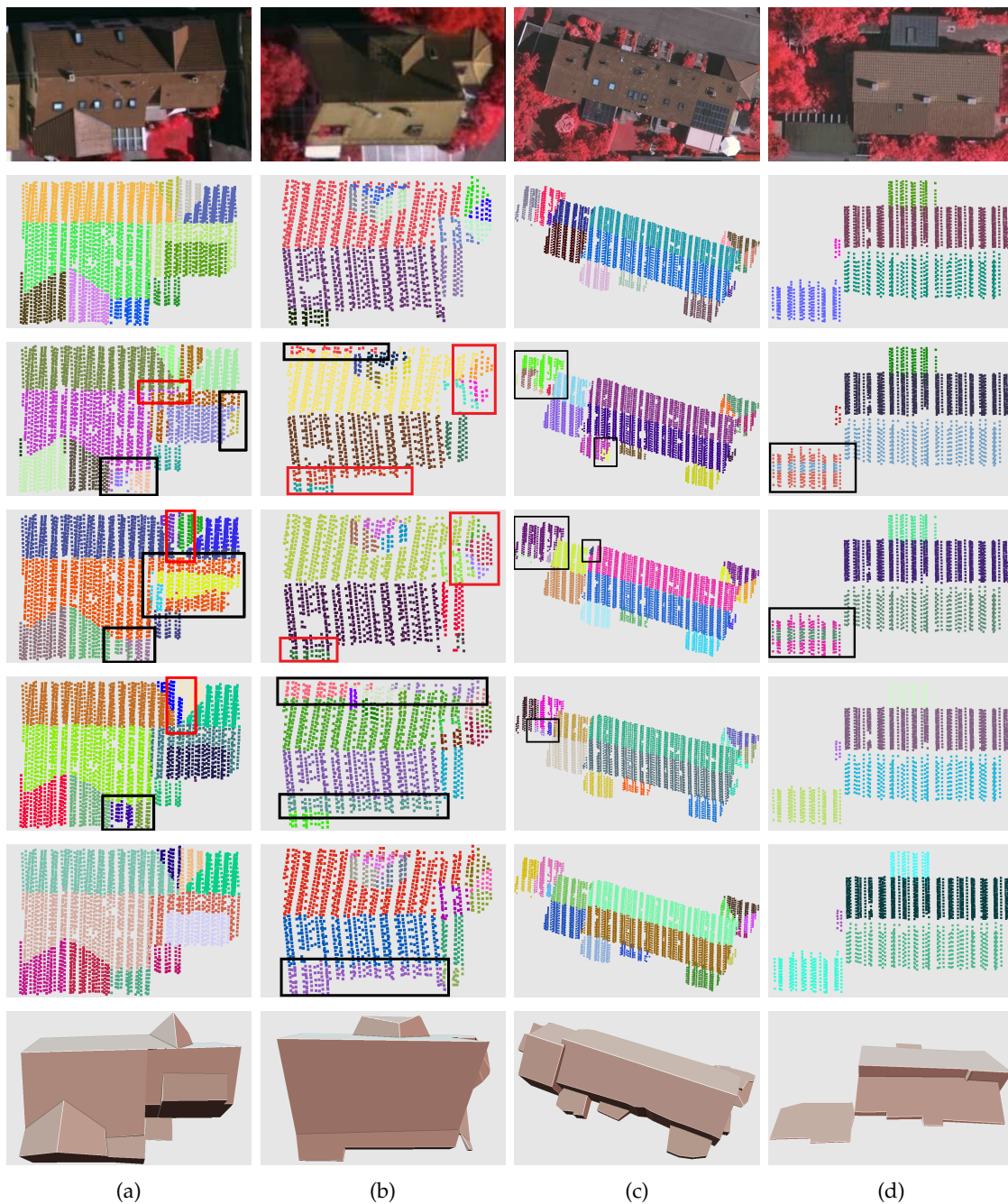
Figure 10. Roof plane segmentation results of different approaches on four local buildings (a–d) selected from the Vaihingen dataset. From the first row to the last row: reference images, ground truth, RG, RANSAC, GO, BR, and 3D models. The black rectangles denote the over- or undersegmentation errors. The red rectangles denote the irregular boundaries.
