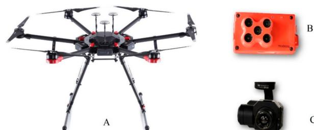
**Figure 2.** UAS platform and sensors applied in acquiring multispectral and thermal images for retrieval of surface SWC. (A) DJI Matrice 600 Pro UAS platform; (B) MicaSense RedEdge multispectral sensor; and (C) DJI Zenmuse XT thermal sensor.
