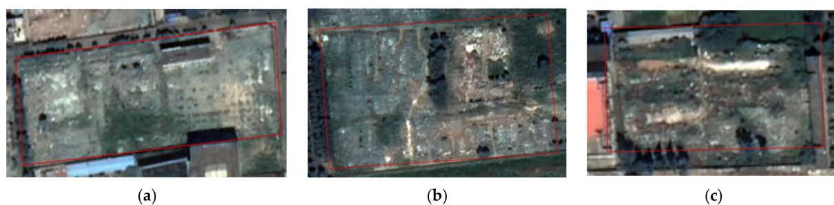
Figure 30. Construction waste covered with vegetation: (a,b) the spectral features of the construction waste, (c) the presence of vegetation in the image object and the use of red bands used to separate vegetation and road at both levels of the classification rules.
