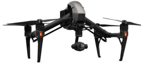
Figure 6. Zenmuse-X4S camera-equipped DJI-Inspire-2 unmanned aerial vehicle (UAV).
