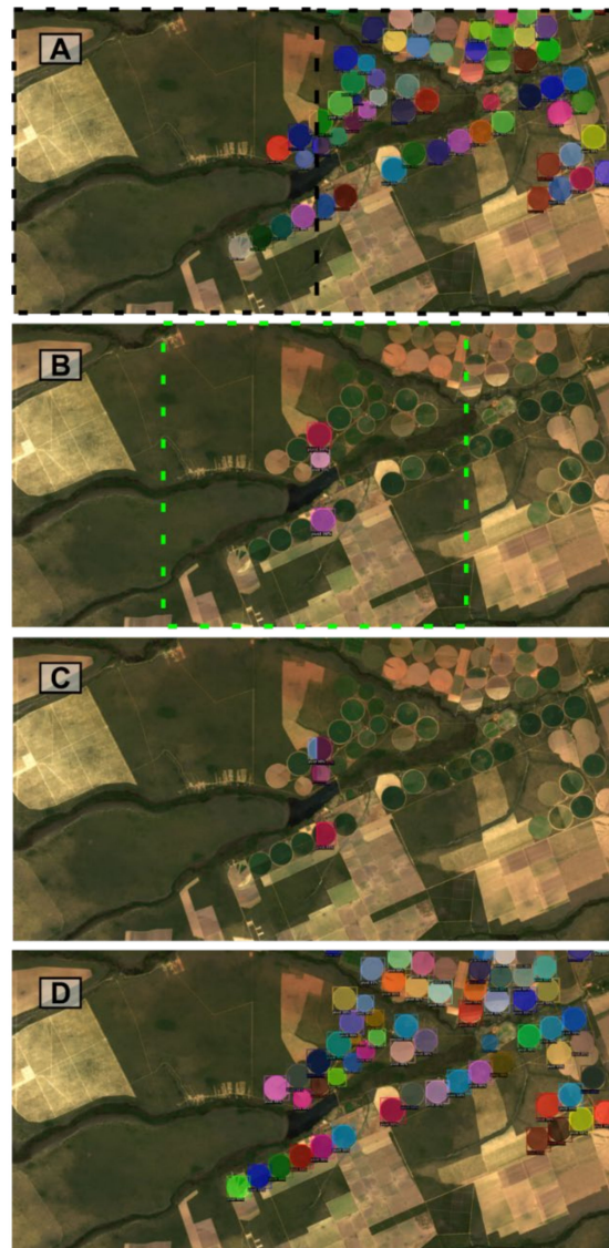
Figure 17. (A) Represents a full classification, (B) represents the horizontal edge classification, considering only elements in the middle, (C) represents the deleted boxes, and (D) represents the final classification.
