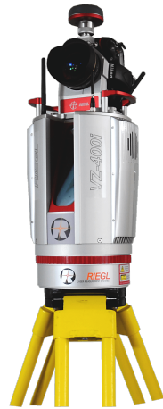
Figure 8. Riegl VZ-400i TLS [61].
