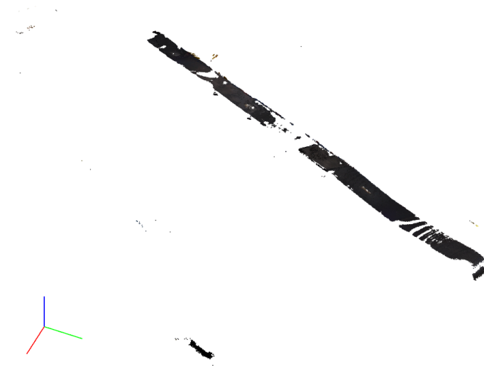
Figure 12. Belt detection enhanced with RANSAC plane fit.
