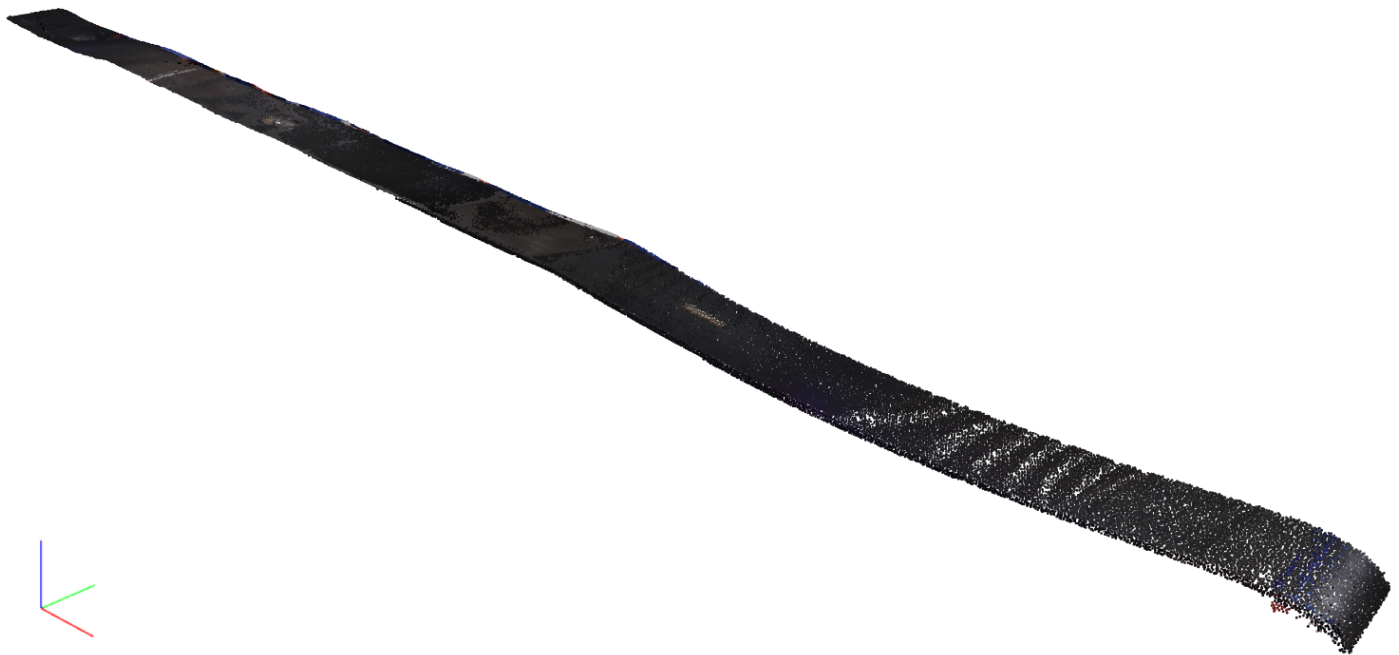
Figure 15. Final point cloud representing the belt surface.
