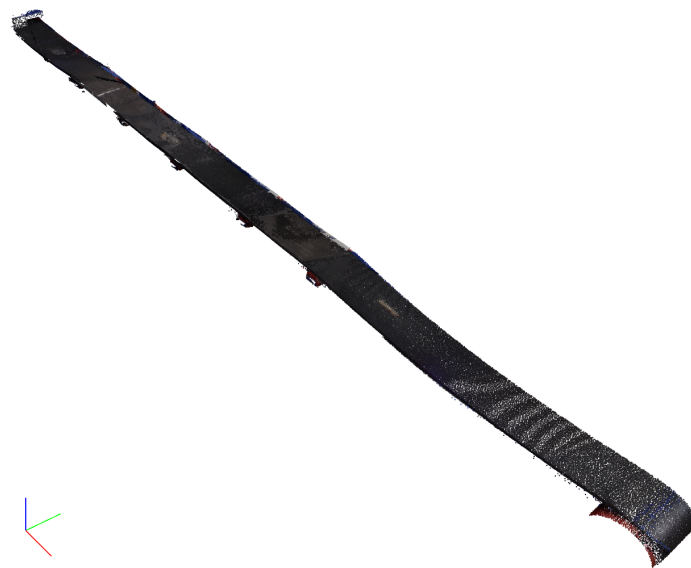
Figure 13. Original point cloud clipped to the belt bounding box.
