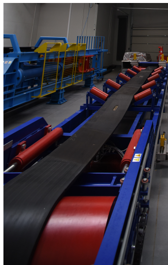
Figure 6. Belt conveyor test rig in GEO3EM Research Center at WUST.
