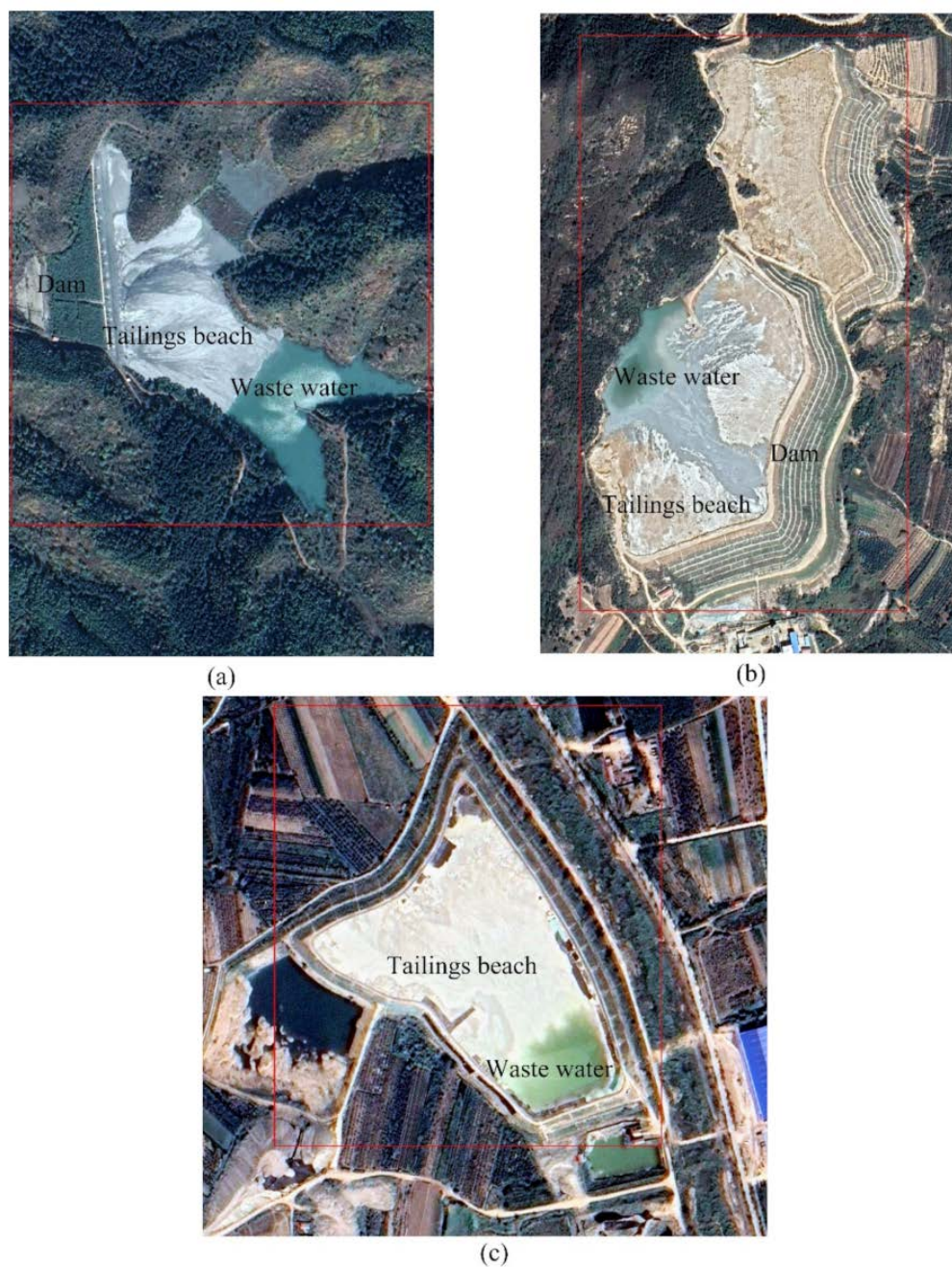
Figure 2. Remote sensing image of sample tailings pond features, with the ground truth bounding boxes shown in red: (a) cross-valley type, (b) hillside type, and (c) stockpile type.
