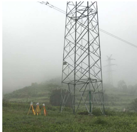
Figure 4. GPS station TB06 under high-voltage transmission line environment (the latitude and longitude of station TB06 are 34^{\circ}08'01'' and 107^{\circ}54'38'' , respectively).
