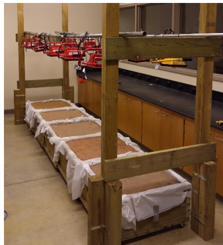
Figure 3. Shows the lab setup of the 5 KRC soils. The soils in order from top left to bottom right: Fine, Coarse, Rink, Stability, and 2NS. Above each bin are two 500 W work lights.
