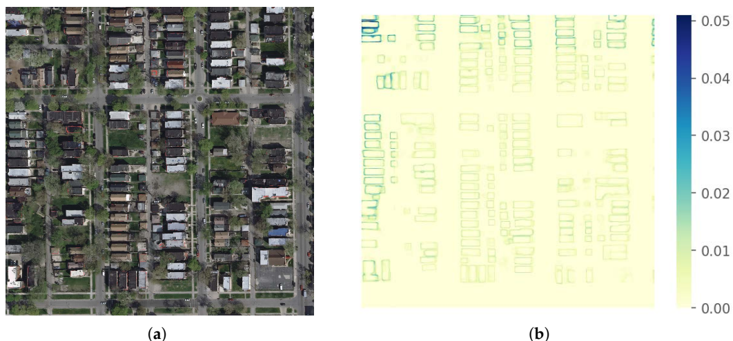
Figure 12. The impacts of the binary geohash can be better recognized by a heat map of the buildings' prediction score. The buildings' prediction scores are the output of the softmax layer within the range [0, 1] . The heat map is obtained by visualizing the absolute values of the difference between the prediction scores of the geohash codes and the zeroed codes. The sample images have a size of 1024 \times 1024 .
