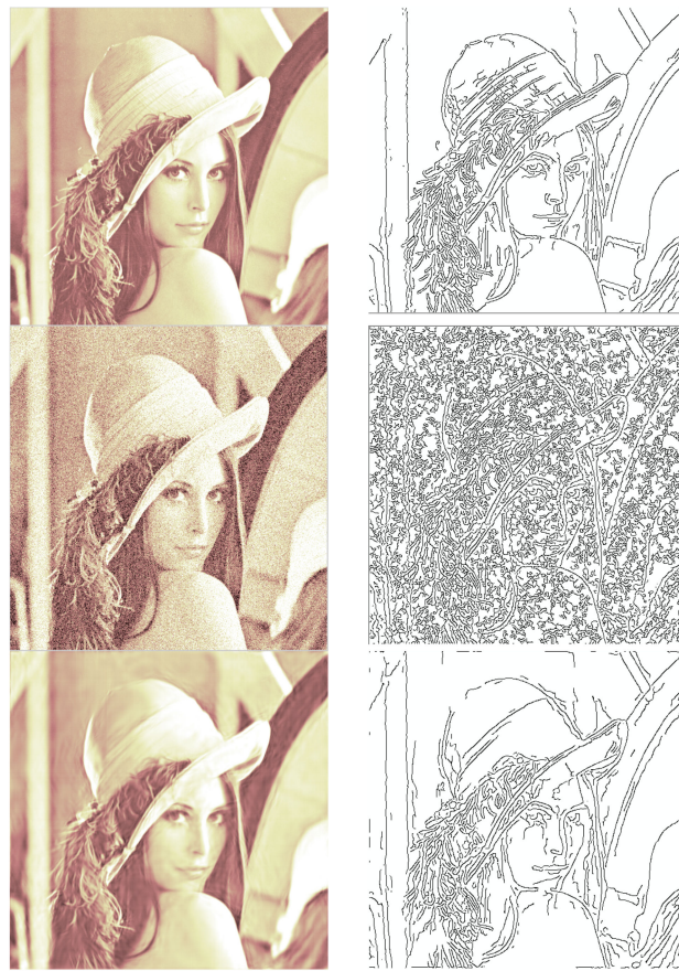
Figure 2. Comparison of results obtained — \sigma_n = 30 . First line: original image and its edge map obtained with Canny’s detector; second line: noisy image and its edge map obtained by applying Canny’s detector; third line: denoised image and the result of the proposed method.
