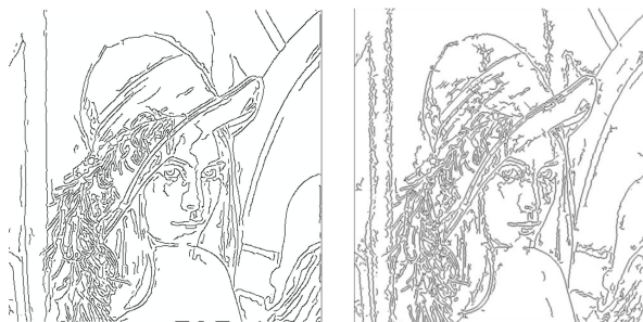
Figure 3. Comparison of the proposed edge detection method and the method in [14] \sigma_n = 15 . The proposed method ( left ); the method in [14] ( right ).
