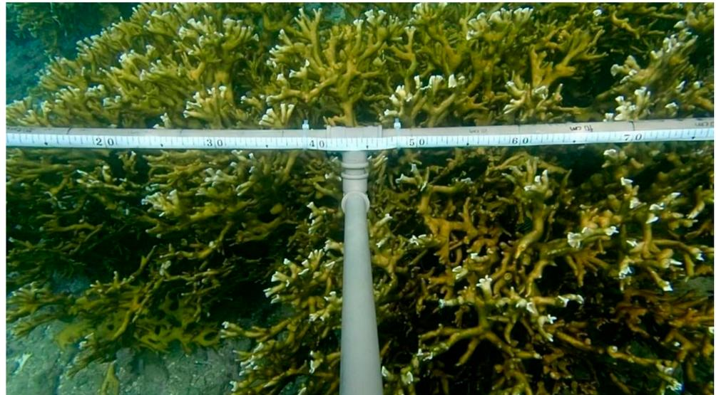
**Figure 3.** Polyvinyl chloride (PVC) apparatus (handle and frame with metric tape) used in the field study to obtain presence records and measurements of *Millepora alcicornis* colonies.
