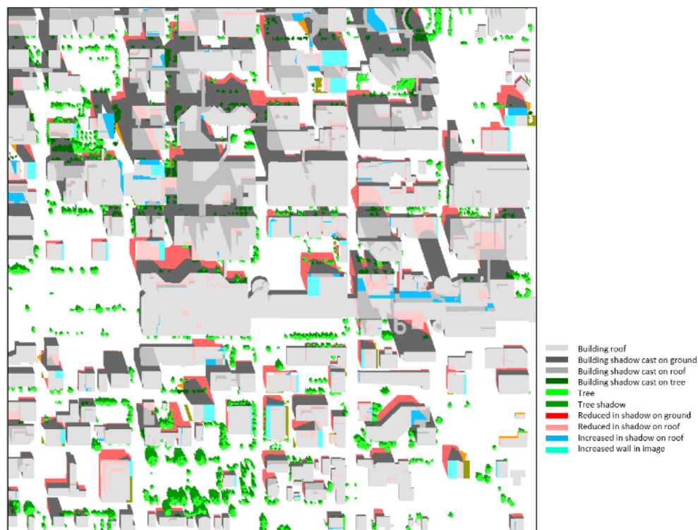
Figure 14. Class map of shadow differences before and after damages derived from building damage case shown in Figure 13.
