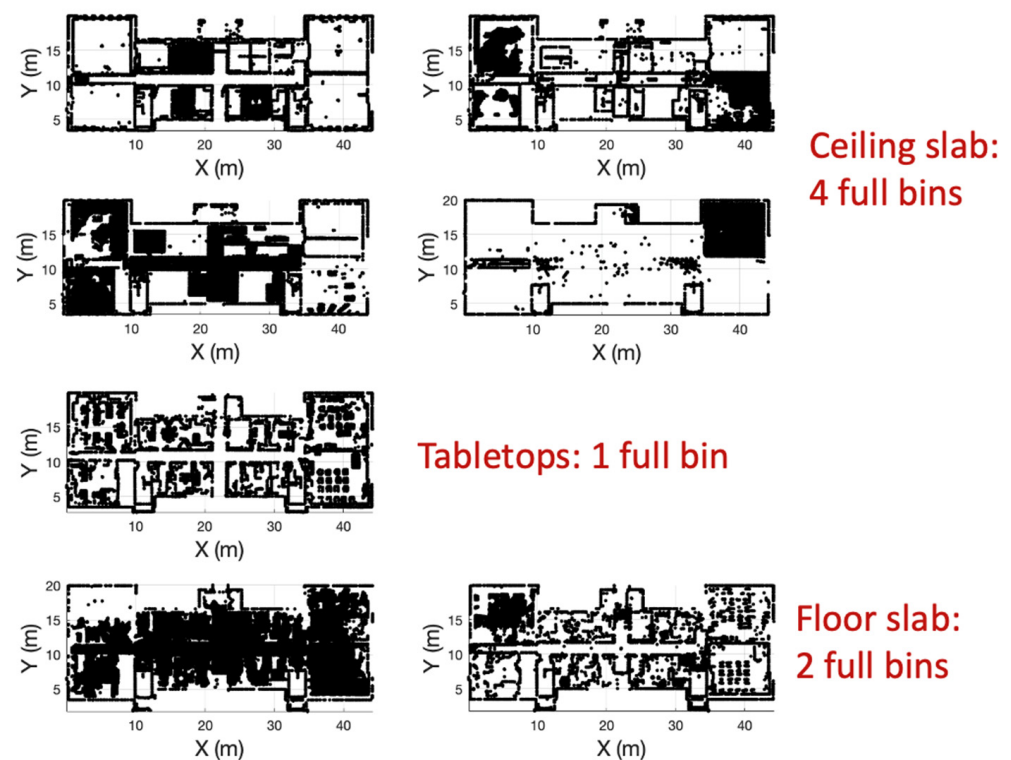
Figure 3. Planar slab examples from the second storey of Old Sun Main Building. The ceiling slab contains four full bins, tabletop returns represent a full bin, and the floor slab contains two full bins. Black represents the portions of the floor and ceiling that were successfully reconstructed, while white represents the gaps in the floor and ceiling slabs.
