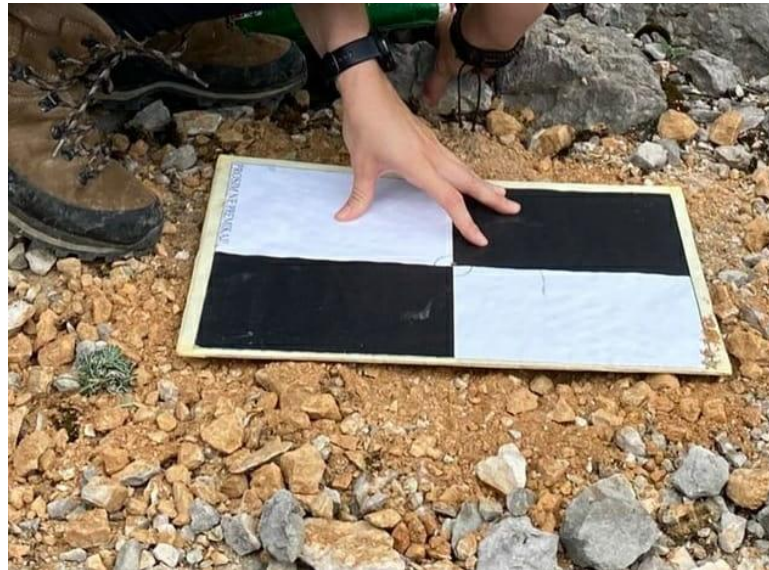
Figure 4. Example of verification point (VP)/ground control point (GCP) target set out in the field.
