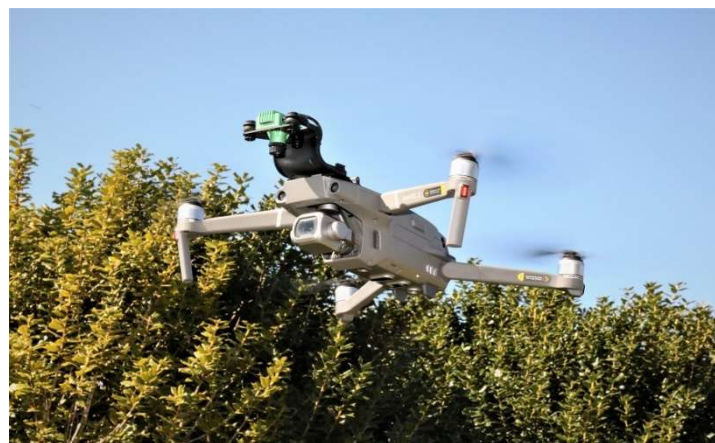
Figure 1. DJI Mavic air UAV with single NDVI camera over the crapemyrtle ( Lagerstroemia spp.) field at Tennessee State University, Otis L. Floyd Nursery Research Center, McMinnville, TN for automatic detection of drought stress in the plants.
