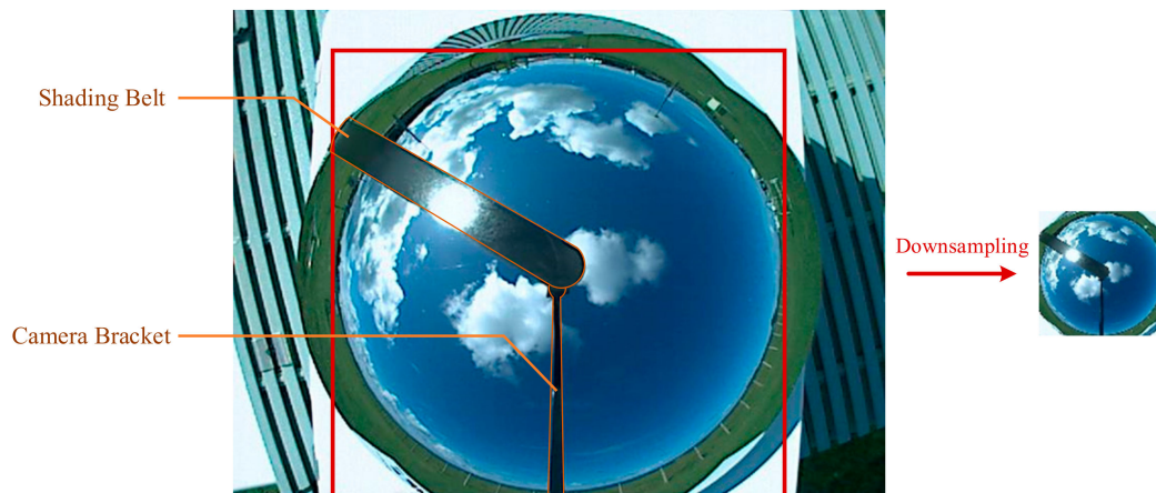
Figure 2. Region of interest (ROI) extraction and downsampling. This is an image taken by TSI-880, including spherical mirror sky imaging, shading belt and camera bracket, as well as ground scenery. The content in the red rectangle is what we need (the region left by clipping, 440 \times 440 ). After clipping, it is downsampled.
