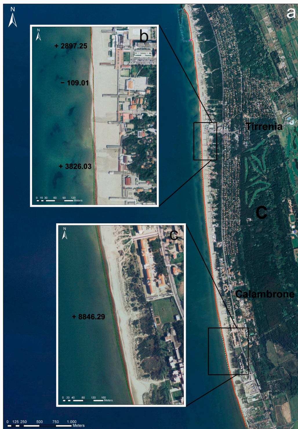
Figure 9. (a) Coastline monitoring in the area C, 23 days after the event of 3 February 2019. Red line DGPS measurements acquired on 1 October 2018, and yellow line DGPS measurements acquired on 26 February 2019. The numbers in (b,c) represent the areal changes (in m 2 ) between the two acquisitions.
