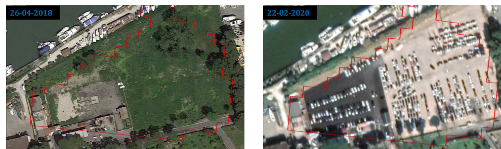
Figure 10. Scene comparison of the Rome Fiumicino airport area. The image on the left has very-high resolution, while the image on the right is acquired by the Sentinel-2 satellite mission. The algorithm correctly detects a new parking area in the scene.
