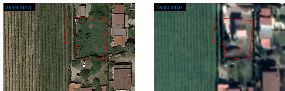
Figure 9. Scene comparison of the Rome Fiumicino airport area. The image on the left has very-high resolution, while the image on the right is acquired by the Sentinel-2 satellite mission. The algorithm correctly detects a new house built in the scene.
