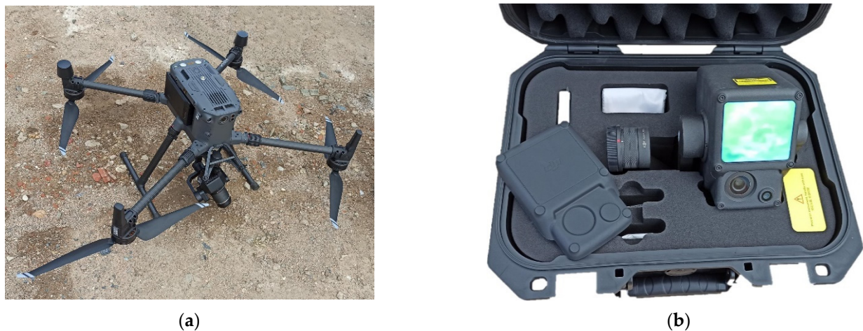
Figure 1. (a) DJI Matrice 300 with a DJI Zenmuse P1 camera (b) DJI Zenmuse L1 in the transport case.
