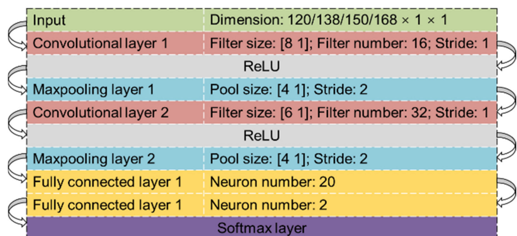
Figure 7. Network architecture of the applied convolutional neural network model.
