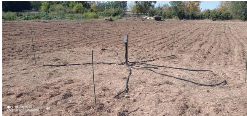
Figure 4. Moisture sensors set up at Test site 1.
