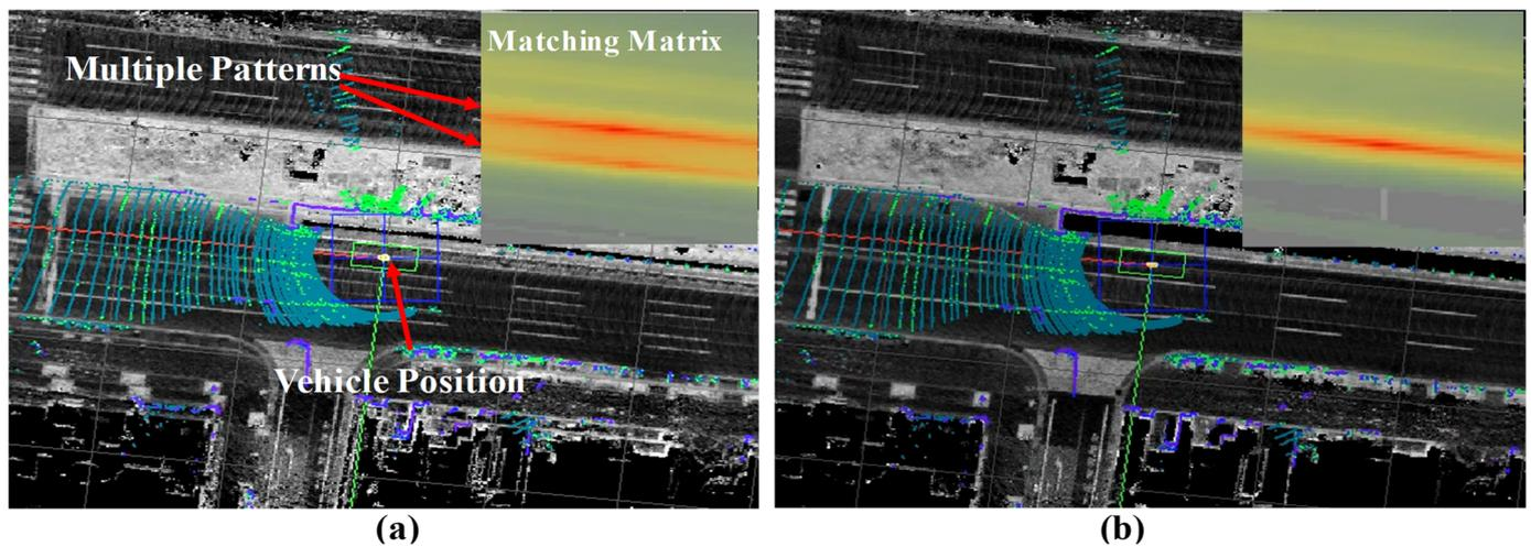
**Figure 1.** (a) Ghosting effects (duplication of road landmarks because of scanning the segment twice with different positioning accuracies by GNSS/INS-RTK) in the map and multiple matching patterns with the observation point cloud. (b) Identical map without ghosting and the corresponding matching result.
