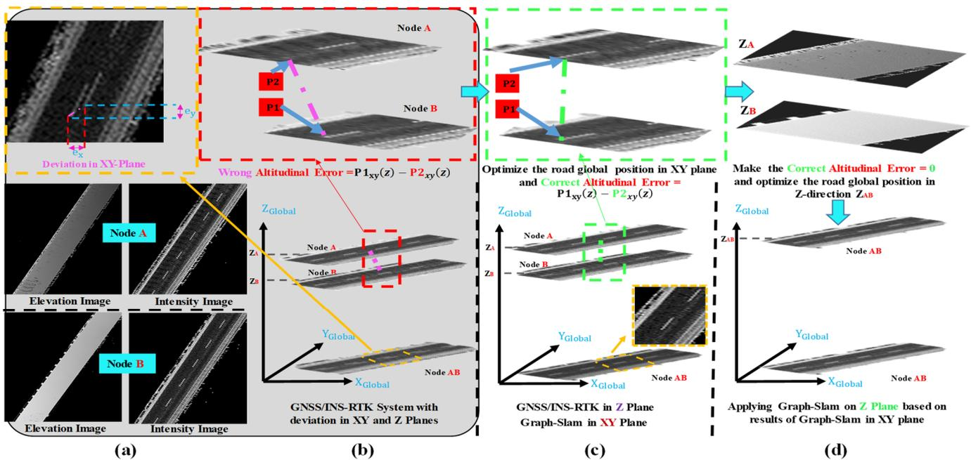
**Figure 4.** Graph SLAM in node level. (a) Two nodes at a loop-closure event with intensity and elevation images. (b) Deviations (relative position errors) between nodes in the XY and Z planes by the GIR system. (c) Applying GS-XY on intensity images by eliminating ghostings and aligning the road perfectly. (d) Applying GS-Z on elevation images using correct calculations of altitudinal errors by GS-XY and making altitudinal errors as small as possible.
