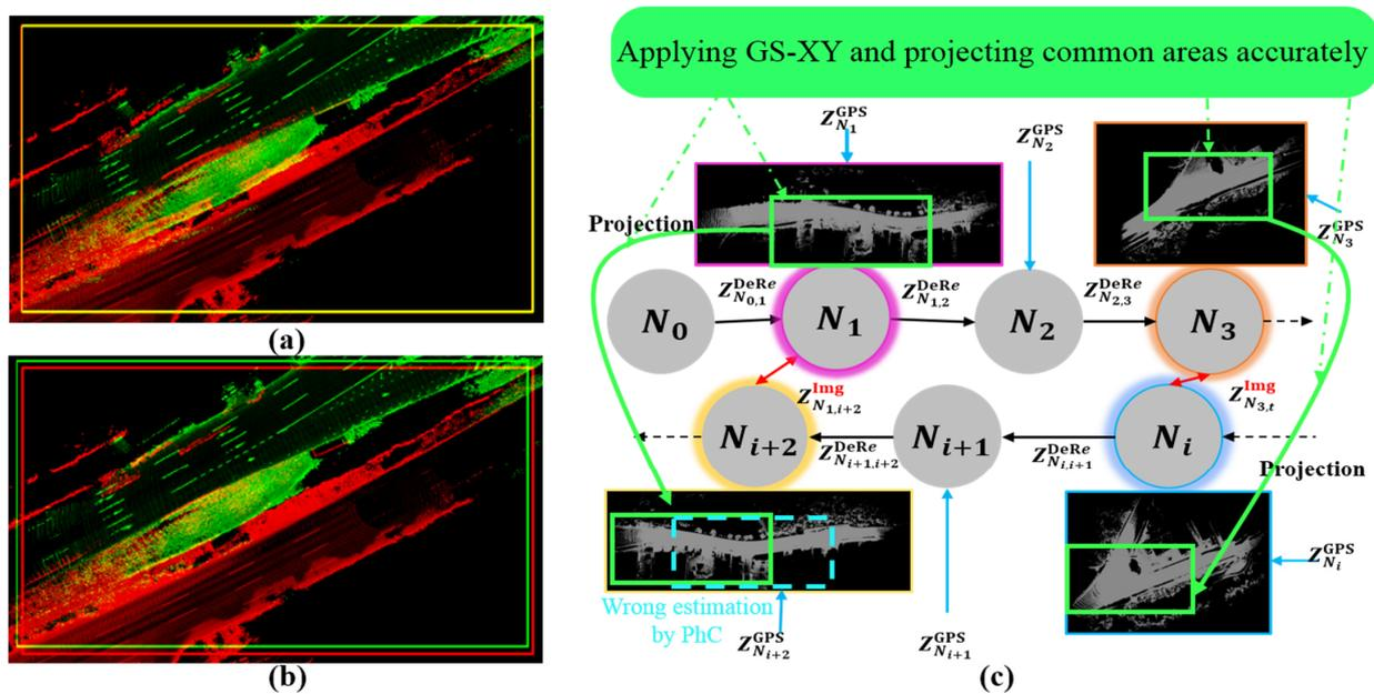
**Figure 6.** (a) Two nodes merged wrongly by PhC. (b) Correct merging by GS-XY showing the correct position of the common area in each node. (c) GS-framework in the Z plane applied on elevation images based on projected areas by GS-XY.
