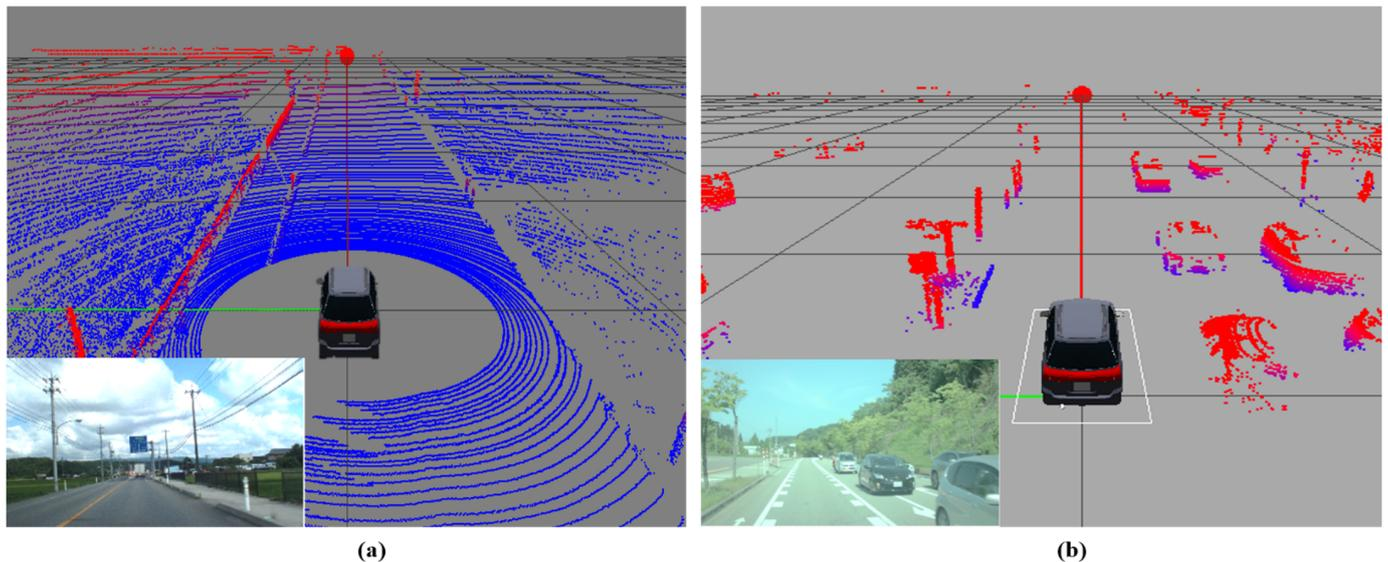
**Figure 2.** (a) Featureless wide road in the Z-direction. (b) Preventing static features to be encoded at a traffic signal by stopped cars.
