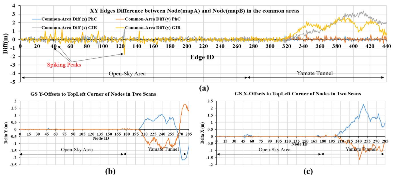
**Figure 9.** (a) Loop-closure edges (coordinate difference) of the common areas between two scans in  $x$  and  $y$  directions obtained by GNSS/INS-RTK system and phase correlation on the node images. (b) The proposed GS-XY's Y-offsets to top-left corners of nodes in the first and second scans. (c) X-offsets to two scans.
