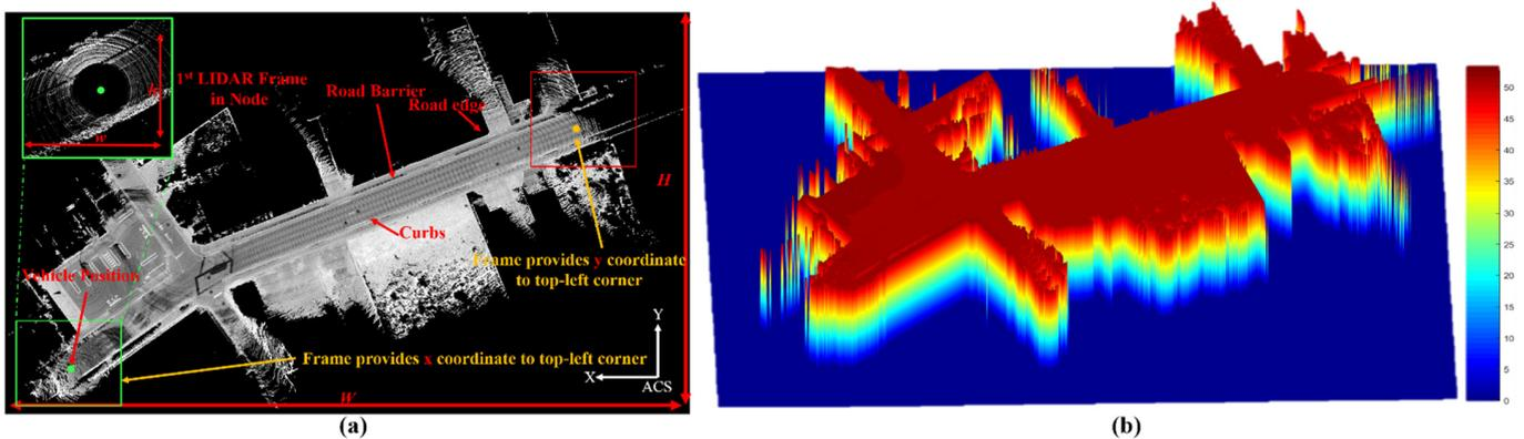
**Figure 3.** Accurate node strategy. (a) Intensity image to represent road surface at 0.3 m in the Z-direction with surrounding environments and top-left corner identification tactic. (b) Elevation image.
