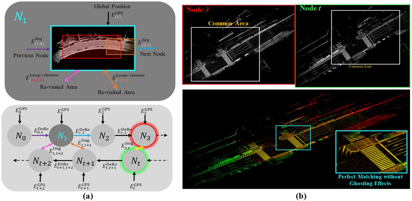
**Figure 5.** (a) Relationship between nodes in the XY plane and edge types of GS-XY cost function. (b) Applying PhC to merge two nodes ( $N_3$  and  $N_t$ ) based on matching road landmarks with estimating common areas for loop-closure edges.
