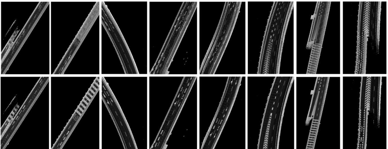
**Figure 10.** Wrong combined node images inside the Yamate Tunnel by GIR (first row) and accurate combination by GS-XY framework (bottom).
