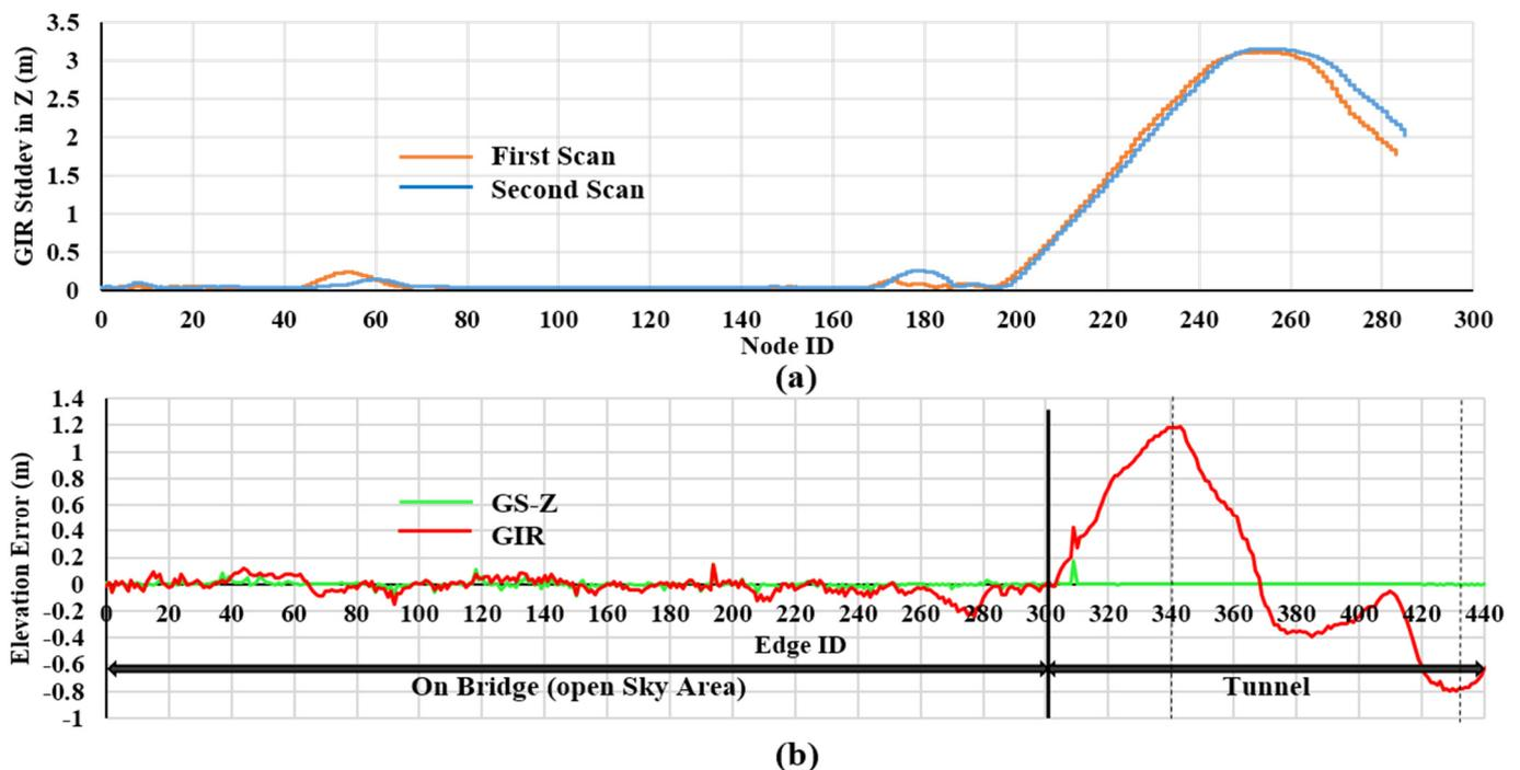
**Figure 12.** (a) Standard deviation of the GIR system in the Z plane showing unstable accuracy along elevation images inside the Yamate Tunnel. (b) Large altitudinal differences between common areas in GIR elevation images (red profile) and the significant small differences after applying GS-Z (green profile). The dotted lines refer to edges in Figure 13.
