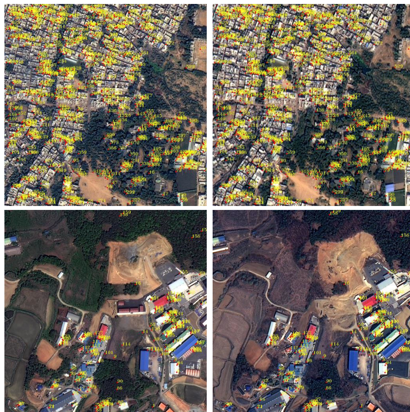
Figure 7. Registered feature points. The images in the left and right columns form bitemporal pairs. The numbered points are the matched feature points in the two images.
