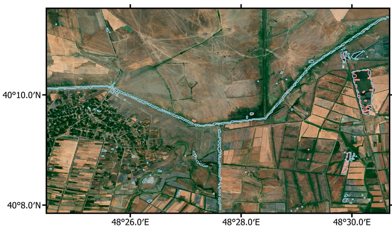
Figure 7. Comparison of the ability of the OPC and JRC methods to detect water in the Bash Shirvan Canal, northeast of Zəngənə, Azerbaijan. The canal water detected by the OPC Max Extent in blue, compared with the canal water detected by the JRC Max Extent in pink. The water body on the east is detected in both datasets, but the canal is only visible in the OPC dataset.
