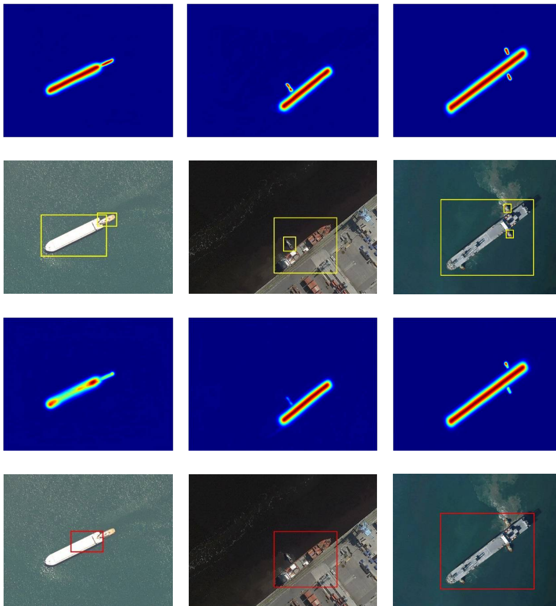
Figure 14. Examples of worse results after using TTA. From top to bottom, the first and second rows represent the ship feature maps and polygon annotations obtained without using TTA, and the third and fourth rows represent the ship feature maps and polygon annotations obtained after using TTA.
