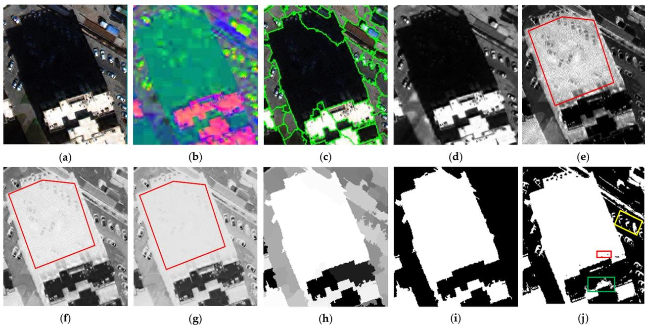
**Figure 3.** Shadow extraction process, where (a) is the original image displayed by RGB bands; (b) is YCbCr model; (c) is the boundary of the mean-shift segmentation result; (d) represents the NIR band; (e) is the  $T_{YCbCr}$ ; (f) is the result of SI; (g) is the result of ISI; (h) is the reconstructed ISI by using segmentation results; (i) is the threshold segmentation result of (h); and (j) is the result of threshold segmentation of (g).
