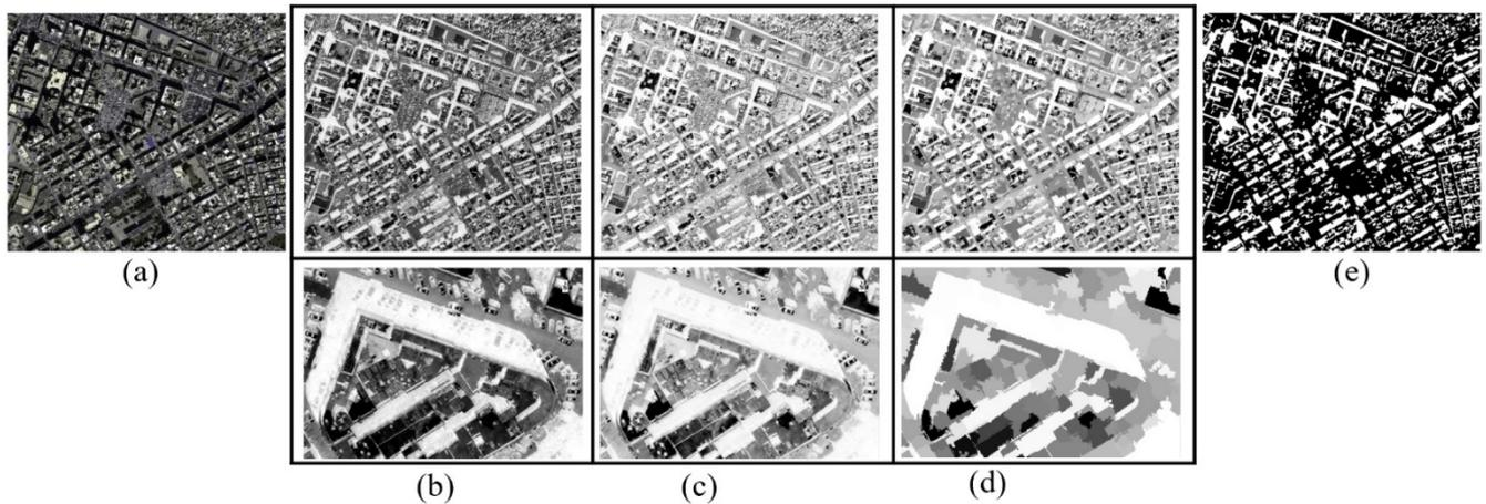
**Figure 10.** Experimental site 2: (a) original image shown with RGB bands; (b) result of shadow detection after threshold segmentation; the first rows of (c–e) are the results of SI, ISI and the reconstructed ISI, respectively; the second rows of (c–e) are the local enlarged view of SI, ISI and the reconstructed ISI, respectively.
