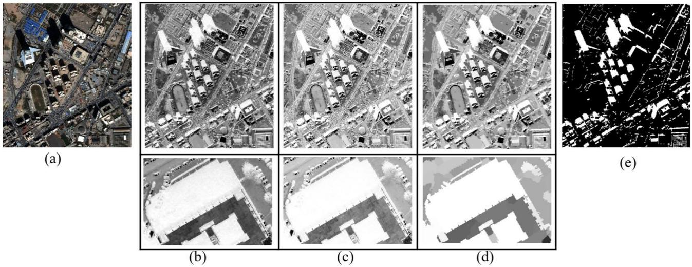
**Figure 9.** Experimental site 1: (a) original image shown with RGB bands; the first rows of (b–d) are the results of SI, ISI and the reconstructed ISI, respectively; the second rows of (b–d) are the local enlarged view of SI, ISI and the reconstructed ISI, respectively; and (e) the result of shadow detection after threshold segmentation.
