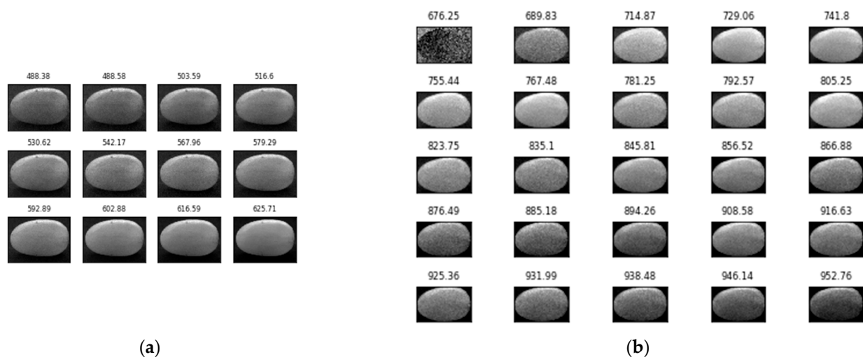
Figure 8. (a) 12 pre-processed bands obtained in the visible spectrum and (b) 25 pre-processed bands obtained in the IR spectrum. The numbers above the images correspond to the wavelength of image acquisition.
