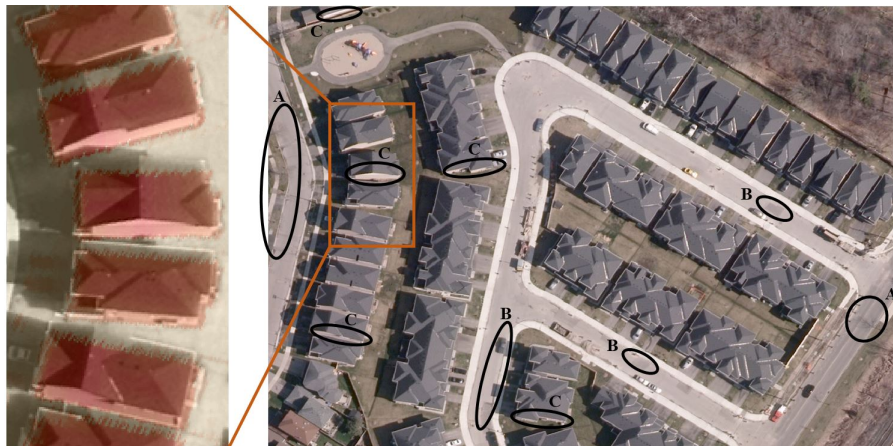
Figure 20. Examples of misclassification by external factors (A: different acquisition time, B: shadow, C: inexact orthorectification) on corresponding aerial photo: the zoom-in shows a height LiDAR-image overlay in transparent orange layer.
