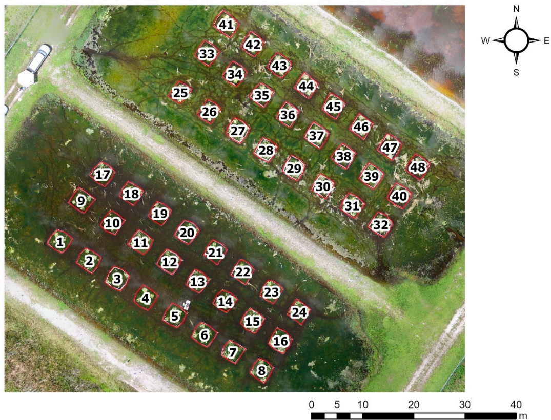
Figure 2. Distribution of 48 treatment plots (TPs) across the north and south test ponds in Stormwater Treatment Area 1 West (STA-1W). The untreated reference TPs are in TP2, TP14, TP33, and TP37.
