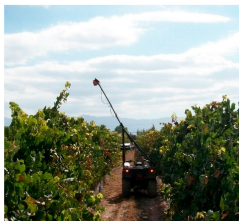
Figure 2. Image collection arrangement. The Tetracam system mounted on a boom and placed in a nadir viewing position over the canopy at each sampling site.
