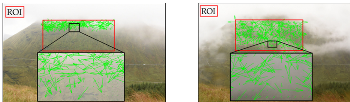
Figure 4. Processing images with cloud generates large number of vectors in random directions. Cloudy images are detected by examining the orientation of these vectors.
