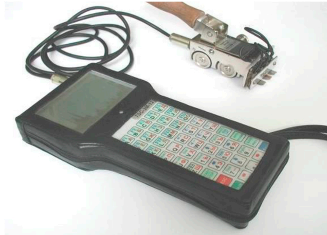
Figure 13. Used device for MMM measurement with an evaluation unit.
