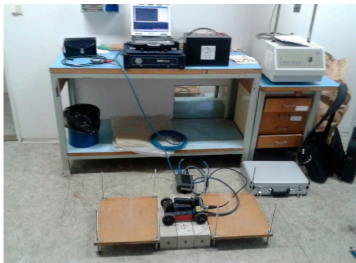
Figure 3. Experimental device set-up of GPR during the test.
