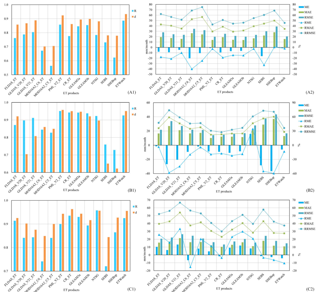
Figure 7. Summary of the assessment indicators ((1) R and d , (2) ME (mm/month), MAE (mm/month), RMSE (mm/month), RME (%), RMAE (%) and RRMSE (%)) for the monthly ET products against the flux EC ET of different climatic zone records ((A) semiarid, (B) dry subhumid, and (C) humid).
