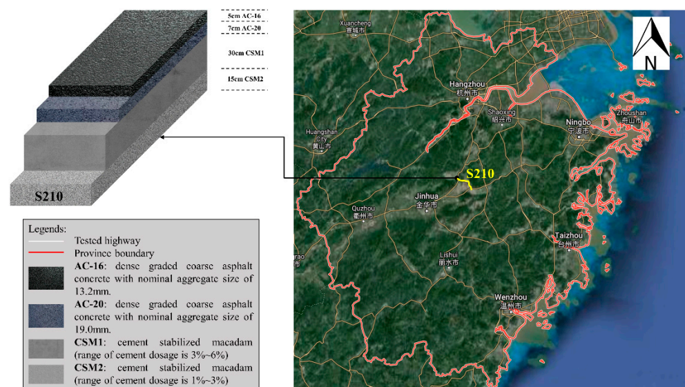
Figure 2. View of the tested road network, construction scheme and materials. The map used is the free version of Google Earth 2020.
