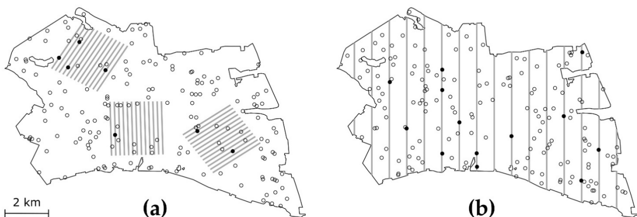
Figure 2. Sample transects (gray lines) under (a) VLOS and (b) BVLOS flight variants with example realizations of a simulated survey of low-density population (two individuals per 100 ha, N = 168 ); open circles represent locations of undetected animals and filled circles represent locations of animals detected with probability p = 0.6 .
