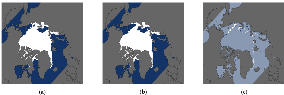
Figure 11. SIE Arctic composites using MWR data from 3 November. (a) FMPL-2 MWR map, (b) Ground truth map, (c) Error map.
