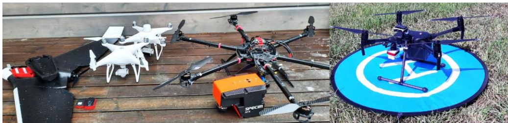
Figure 2. Four types of unmanned aerial vehicles (UAVs), shown from left to right: (1) fixed-wing Parrot Disco and Parrot Sequoia multispectral camera; (2) DJI Phantom 4 and Phantom 4 Multispectral RTK; (3) custom-built Carboncore hexacopter and Specim AFX10 push-broom hyperspectral camera; and (4) DJI Matrice 210 with Micasense Altum multispectral camera onboard.
