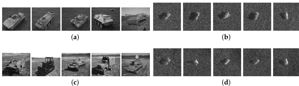
Figure 8. Optical images and MSTAR SAR images of targets. (a,b) optical images and their corresponding SAR images for BMP2, BTR70, T72, BTR60, 2S1; (c,d) optical images and their corresponding SAR images for BRDM2, D7, T62, ZIL131, ZSU23/4.
