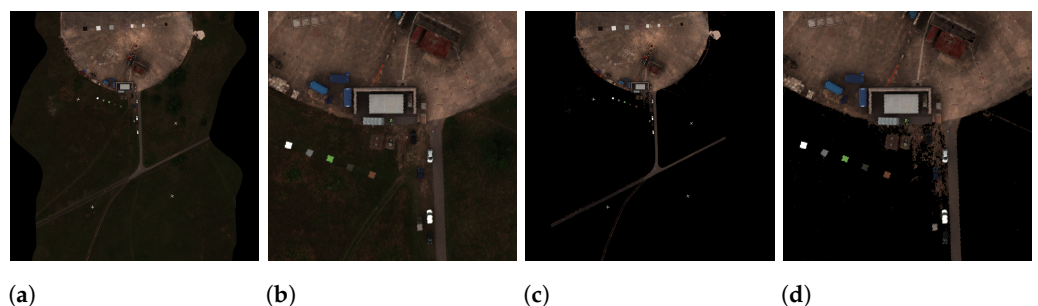
Figure 14. Example image from the UDRC Selene Dataset. (a) False colour image of the target area. (b) Enlarged version of (a). (c) Retained pixels following the NDVI_{re} spatial masking. (d) Enlarged version of (c).
