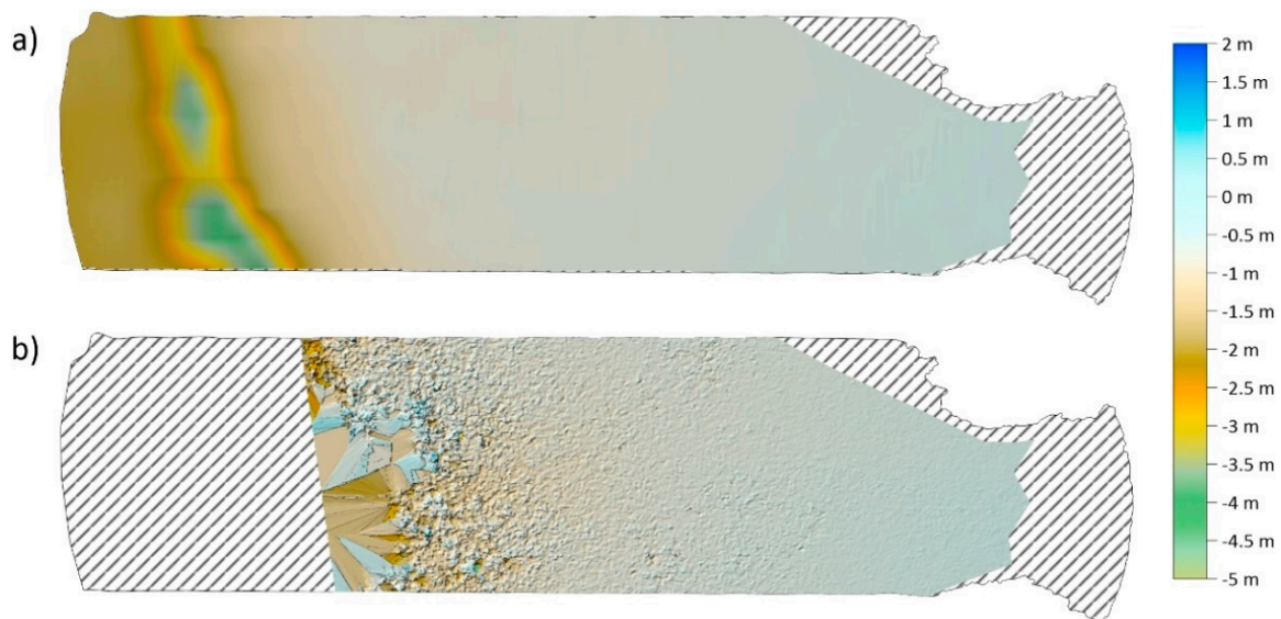
Figure 9. BRS surface developed by the TIN method from USV data in the sounding domain (a) and the corresponding surface developed from UAV data (b). View within the limits of the complete development of the digital bathymetric model.
